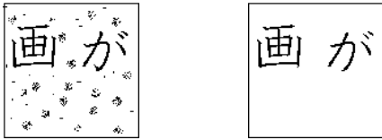
(a) Input image 120 \times 120 pixels (b) Noise removal with EPS = 6
